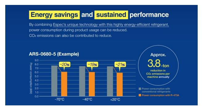
We are pleased to announce the release of the new Refrigerant R-473A for Espec environmental test chambers. This new refrigerant can be ordered as an option to replace R23 and R-508A. R-473A is an environmentally friendly low GWP refrigerant that has cleared regulations globally. Its characteristics make it possible to reduce both power consumption and the amount of refrigerant required.
