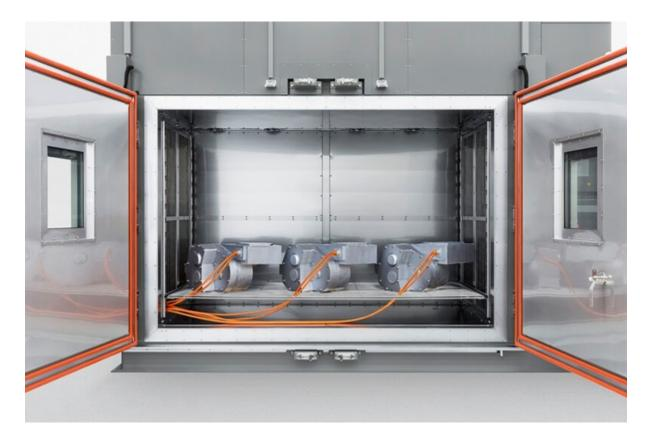
Rapid advances in automotive electronics technologies have lead to an increase in demand for test chambers that are capable of testing these devices. Espec TSA Series, large capacity thermal shock chambers, meet these demands offering accurate, extreme environmental simulation to support cutting edge technology.
