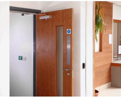
It is non-handed for right and left swinging doors and features adjustable hydraulic backcheck to cushion the opening swing prior to 90 degrees. There is separate regulation of the general closing speed and the latching speed. The LCN 1261 carries UK Fire Certification in accordance with BS EN 1634-1:2014 (timber) - 120 mins and is CE Certified.
