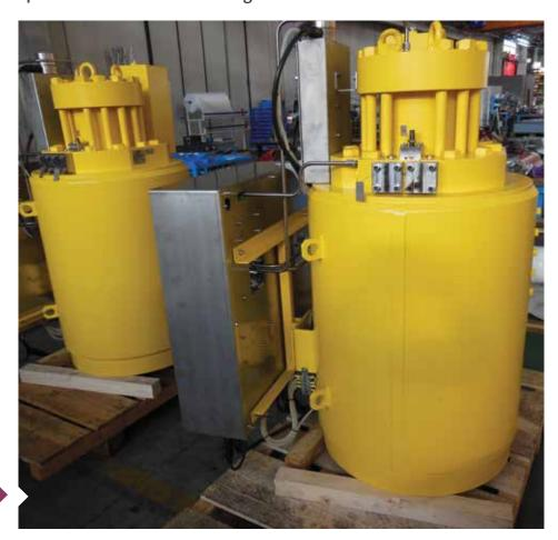
The innovative configuration of hydraulic cylinders, quick exhaust valves, flow regulators and internally mounted discharge ports provides an extremely compact and reliable actuator solution with significant reductions in associated piping.
