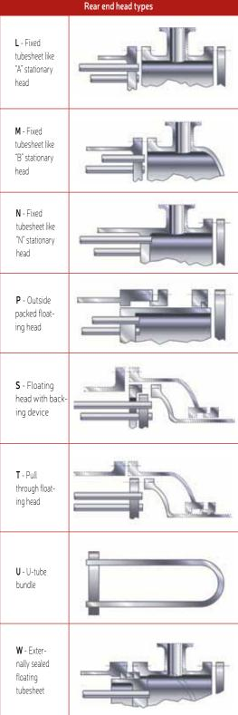
★ The typical TEMA type heat exchangers listed in the table can be visualised from the diagrams shown here (right and left). From the three-letter coding for each type of exchanger (AEW, BEW, AEP and so on, as listed in the table) a picture can be built up of the final shell and tube assembly of front- end stationary head, shell type, and rear-end head
