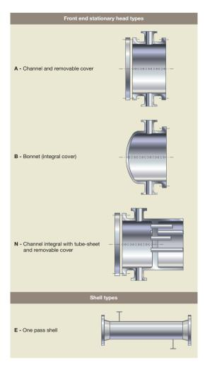
The typical TEMA type heat exchangers listed in the table can be visualised from the diagrams shown here (right and left). From the three-letter coding for each type of exchanger (AEW, BEW, AEP and so on, as listed in the table) a picture can be built up of the final shell-andtube assembly of frontend stationary head, shell type, and rear-end head
