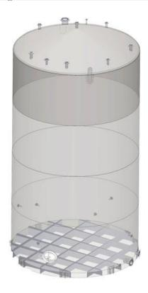
As part of a staged repeat order we have supplied 2-off 125,000 litre stainless steel bulk storage vessels. The tanks were designed in line with EN 14015 and manufactured in house with an interlocking flat sloping base.
