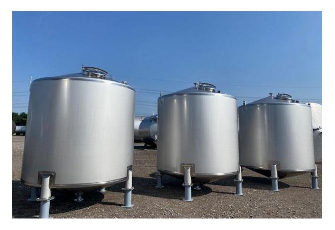
This week we saw the first 5 of 30-off stainless steel 316, low profile tanks we are supplying one of Europe's largest lubricant manufacturers leave site. They will be installed in Shrewsbury at our customers production site. Once completed, the project will total 260,000 litres of hygienic lubricant storage.
