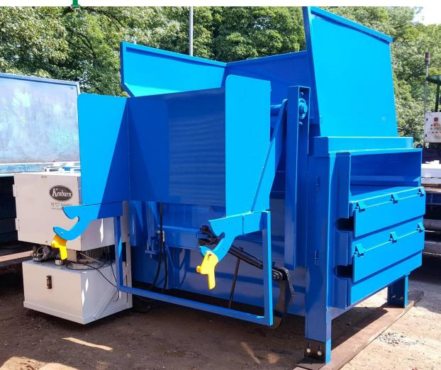
A compactor is a machine that's used to compress and compact materials and can be either portable or static.
