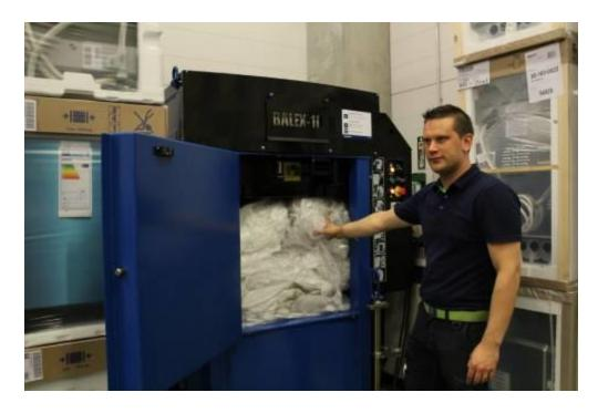
Plastic waste balers have the benefit of increasing efficiency in several different ways, including reducing employee workloads, saving labour costs and preventing workplace injuries, while streamlining the process compacting and recycling plastic waste.
