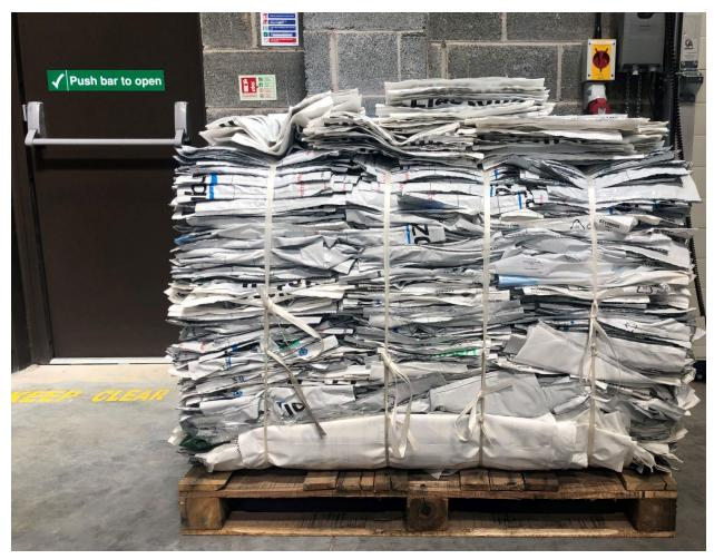
The plastic mode can also be adjusted to compact various types of soft and rigid plastics, so with thermoplastic polyurethane, the compaction cycle can be programmed to create heavy dense bales by slowing down the compaction cycle time.
