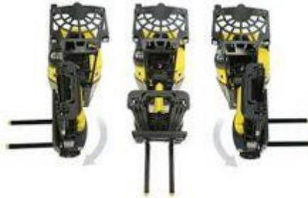
These VNA articulated pivot trucks are often know as Flexi or Bendi (the manufacturers' name). And VNA? It means Very Narrow Aisle. The space between each of the lengths of racking (shelves) is called an Aisle.
