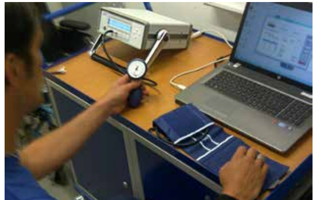
In practice: Blood pressure monitors in the nursing home Solina in Spiez (Switzerland) are calibrated by the technician responsible.
