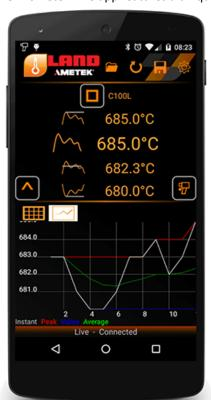
recorded at pre-configured locations. Single or multiple routes can be uploaded onto the app, with the option to preset against a variety of parameters such as emissivity and window correction.
