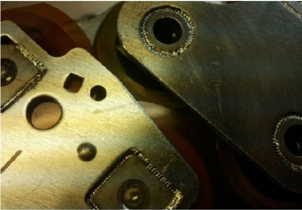
Pulsed laser welded interconnects
