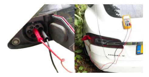
Rated at 1000V CAT III/ 600V CAT IV 12A IEC61010, you can be sure in knowledge that the test lead meets the safety standards required to keep risks to as low as reasonably practical.
