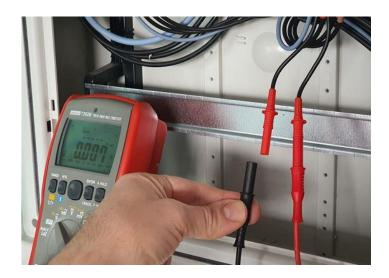
The <u>AdaBV140</u> consists of a 2.50mm<sup>2</sup> insulated flexible solid copper conductor and shrouded 4mm Banana socket with a finger guard to protect against inadvertent touching of a conductor under test. The 4mm socket enables connection to common electrical test and measurement equipment such as multimeters, power analysers, insulation testers and oscilloscopes.
