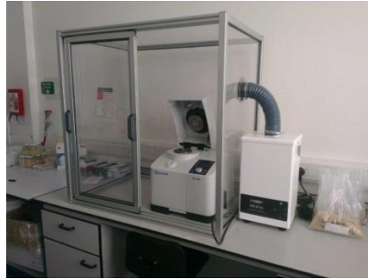
Fume extraction cabinet
