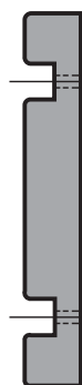
1 WALL GUARD Standard Length 3000mm Material EPDM Rubber Fixing Method 'Hammerfix' anchors (13 No.) c/w Cup Washer @ 500mm Centres
