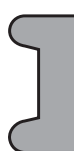
3 DOUBLE 'D' Standard Length 6m Coil Material EPDM Rubber Fixing method 'Hammerfix' anchors (or similar) c/w Washer @ 400mm centres
