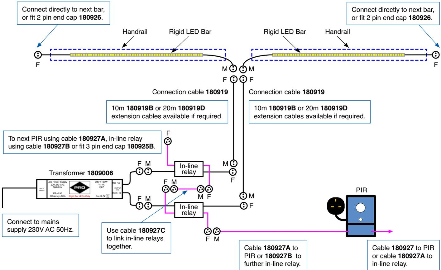
More than 6 pieces of 850mm, or 12 pieces of 425mm, long white, or single colour rigid LED bar. Single or multiple PIR controlled.
