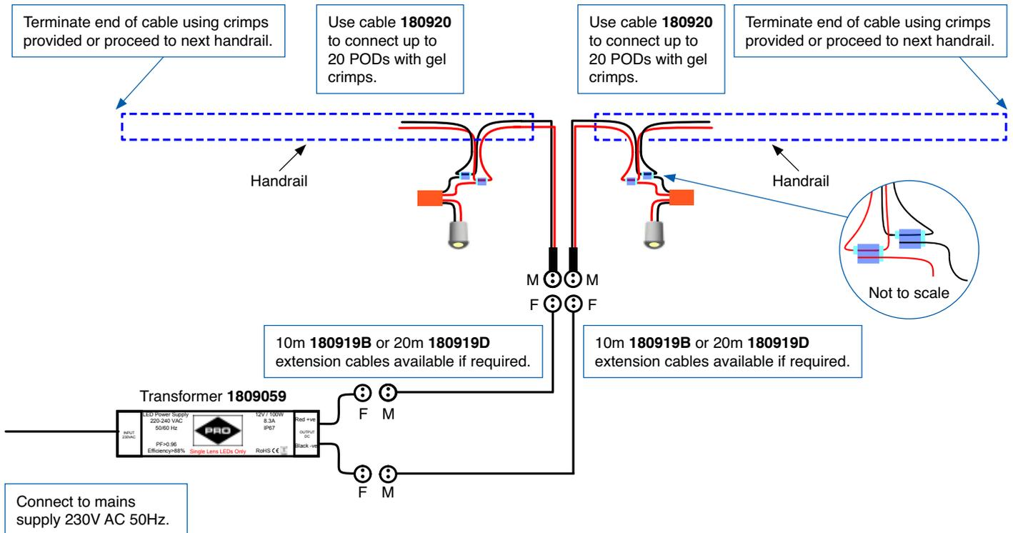
Single Lens System. PIR(s) operation. Up to 40 LEDs.
