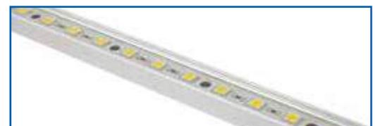
LED bar is a sealed one piece unit rated to IP67, with 54 LEDs totalling 12.24W. With a brightness of 3000K. They are supplied with a 200mm cable with waterproof connectors.
