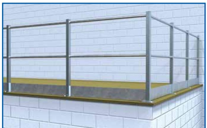
The system is supplied with BZP square RHS posts, tube and galvanised flat bar kick plate to conform to BS 4592-0:2006+A1:2012 requirements.
