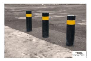
The Resilience SSF100 bollard was physically tested in an array of 3 bollards to the IWA 14-1:2013 impact test using a N2A 7200kg vehicle travelling at 64kph.
