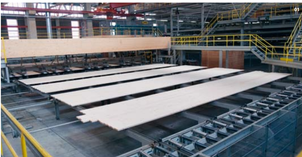
01 The CLT elements are transported on a roller table with cross-transfer conveyor to the MAKa machine.
