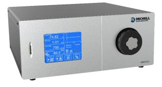
The new Michell S8000 RS is a high-precision, low dew-point hygrometer designed to meet the demands of humidity calibration laboratories and industrial applications. Michell's engineers have used the latest developments in chilled mirror technology to achieve reliable, repeatable measurements of low frost points down to -90 °C, with an accuracy of  $\pm 0.1$  °C, without the need for additional cooling.
