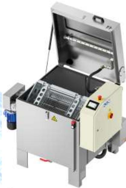
The new Teknox Twister is an ideal washing system for spray washing multiple small components contained in a preloaded detachable stainless-steel basket.
