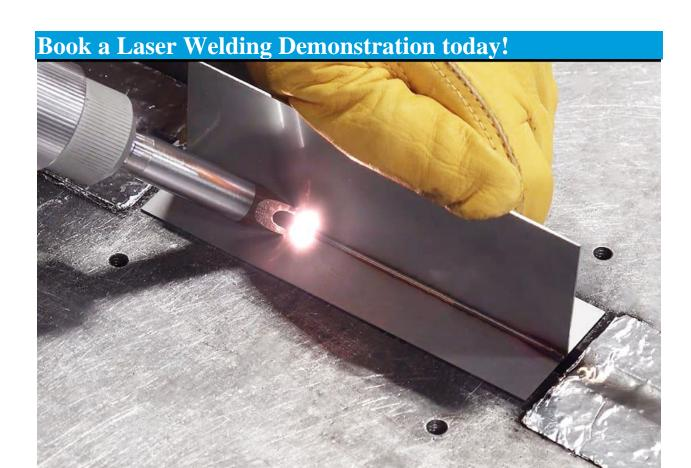
Laser Welding is the latest innovation in welding, offering speeds up to 4x faster than TIG, and far easier for an unskilled worker to pick up and learn to use than the alternatives. It creates, strong, stable welds across a multitude of materials.
