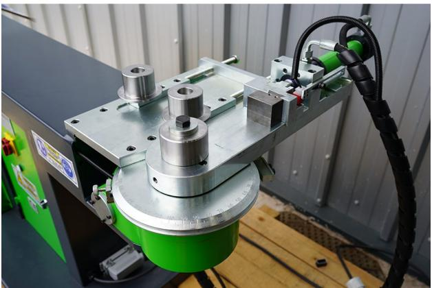
Assorted tooling allows you to handle either solid, or hollow tubes, for forming into bow tops.
