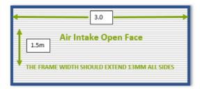
Note: If the equipment or air intake you are attempting to attach to is not flat surfaced 12 mm outside of the actual filter face, you should expand your measurement until you can mount your frame on a flat surface. Add this to your filter measurements. We have alternative border and fixing options available if this is an issue.
