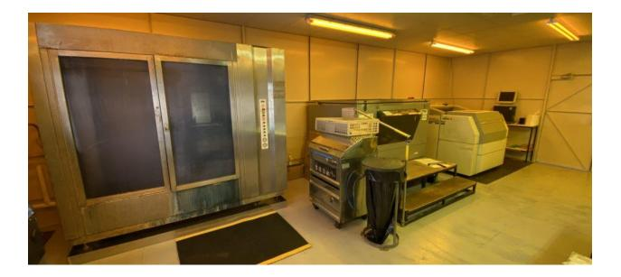
Our in-house pre-press department is a crucial cog in our manufacturing process, where the customer's artwork is exposed to a photo-sensitive polymer. Then the polymer on the screen material is washed out to create negative space for screen printing inks to pass through onto a substrate material. Having this on-site department means there is always an immediate response to any print issues.
