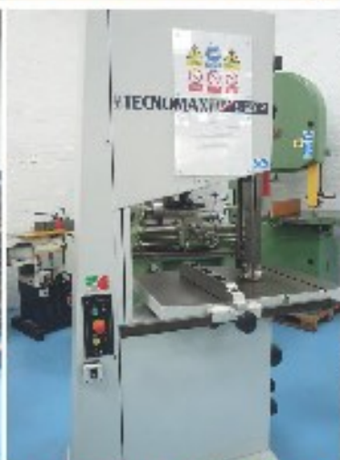
SCM Centauro Technomax S 600P Vertical Wood Cutting Band Saw £2,750.00 580mm Throat, 360mm Under Guides, 580 x 810mm Tilting Table, 600mm wheels
