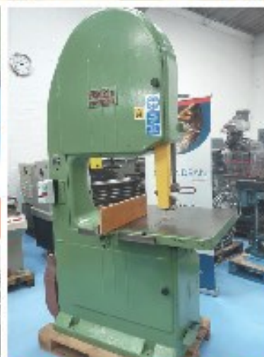
Wadkin 3082B Vertical Wood Cutting Band Saw £4,750.00 710mm (28") Throat, 355mm (14") Under Guides 760 x 760mm (30 x 30") Tilting Table
