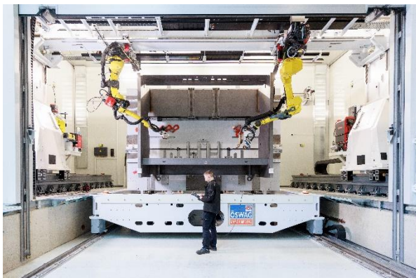
Gantry welding system with two welding heads—LaserHybrid and MAG—from Fronius International. Equipped with two tilt positioners for setup parallel to production. Components are moved in by motor.
