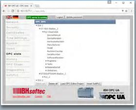
A microSD card with the OPC UA server/client with IBHsoftec firewall is available for the Siemens Gateway IoT2040 (6ES7647-0AA-00-1YA2). By simply plugging the preconfigured microSD card from IBHsoftec, the IoT2040 becomes an OPC UA server/client for Siemens PLCs. This solution integrates SIMATIC S5, S7-200, S7-300, S7-400, S7-1200, S7-1500 and Logo! (Ethernet versions) Controllers into the OPC UA world.
