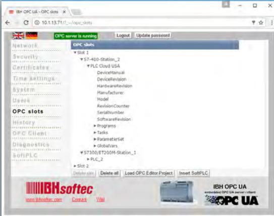
A microSD card with the OPC UA server/client with IBHsoftec fire-wall is available for the Siemens Gateway IoT2040 (6ES7647-0AA-00-1YA2). By simply plugging the preconfigured microSD card from IBHsoftec, the IoT2040 becomes an OPC UA server/client for Siemens PLCs. This solution integrates SIMATIC S5, S7-200, S7-300, S7-400, S7-1200, S7-1500 and Logo! (Ethernet versions) Controllers into the OPC UA world.
