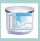
1 This touch free waterless patented urinal cartridge is made out of non-stick, non-porous material and designed to work like a funnel. Urine passes through the waterless system where the Falcon Waterfree Technologies' sealant forms a barrier between it and the washroom space.
