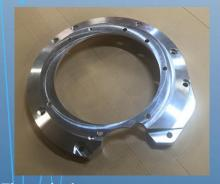
Central Engineering then programmed one of their fleet of high precision CNC machining Centres to produce this component in only (6) hours!
