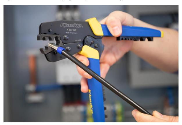
We've all come across the situation where bootlace ferrules don't seem to grip the cable enough and in worst case can be pulled off. This in the main is due to the crimping profile of traditional ratchet tools being of a fixed dimension. When a cable is slightly smaller in physical diameter, there is less material in the ferrule and the fixed tool profile doesn't compress it enough.
