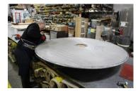
New meshes are then measured, cut and spot welded to the clean frame, ensuring that the mesh sits evenly across the frame.
