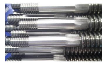
We also have a state of the art <u>Ball Screw Softening</u> machine at Moore International which allows us to anneal the hardened Ball Screw shaft for easy machining, we also offer this softening facility on all the Ball Screws we supply so if you do have machining facilities you can machine your new <u>Ball Screw</u> with ease.
