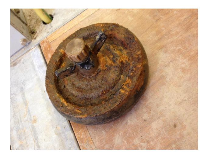
Mechanical bung removed from a leaking duct.....
