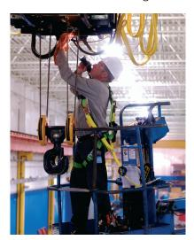
preventive maintenance program that uses a multi-point visual inspection to capture data on the condition of over 225 crane components. The data is then used to create a customized plan for scheduled maintenance and repairs. Konecranes currently conducts annual MAINMAN<sup>®</sup> inspections at the facility and completes scheduled preventive maintenance repairs as needed.
