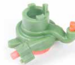
Wax master with soluble inner core (length 75mm, height 54mm)
