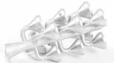
Tree assembly as cast (length 255mm)
