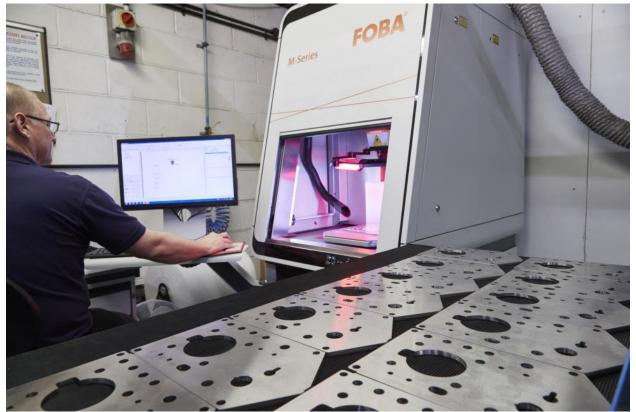
We provide a range of laser engraving and etching sub-contract services which are used to accurately and permanently mark the surface of materials with high-quality text, lines and logos.
