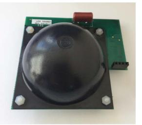
The Euro-Gas Radon SS sensing component detects field range of 0-65,000Bq/m3 levels. With a uniquely designed high performance phototransistor sensor, it has a standard range of 1750pCi/l Rn. Its easy-to-use advanced technology makes it an ideal sensor for installation into both portable and fixed detection equipment in air quality and gas detection, delivering a complete set of information for instantaneous and average Radon alpha particle concentrations.
