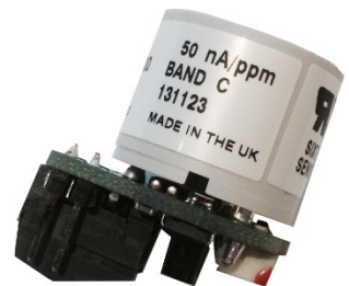
ECO-Sure sensor with 4-20mA circuitry
