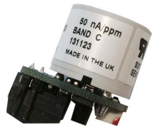
ECO-Sure sensor with 4-20mA circuitry
