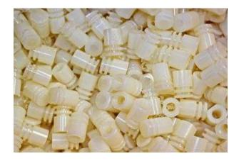
A typical batch of plastic turned parts. Cycle times vary from around 15 seconds to several minutes and almost all parts are produced in the subcontractor's lathes in one hit.
