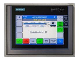
The Siemens touch-screen control fitted to the Boss barfeed has three standard programs, including one for use when smaller diameter plastic bar is being supported by and fed through the bespoke clamping blocks.
