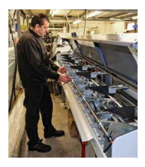
Fitted to a Cincom 12 mm capacity sliding-head lathe, this lemca Elite bar magazine can be changed over in seconds from gravity feed to walking-beam advancement of the bars.
