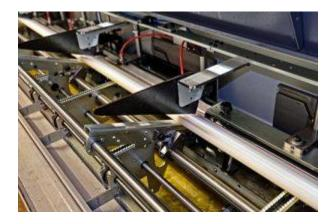
The lemca Elite in gravity feed mode.
