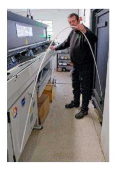
An Iemca Boss 338-HD superfast barfeed is fitted to this 20 mm capacity Cincom LFV lathe. Darren Evans shows that even 12 mm diameter PTFE behaves like spaghetti.
