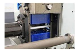
Additionally, the Italian manufacturer fitted clamping blocks to the end of the bar magazine to ensure that smaller diameter stock enters the turning centre horizontally.
