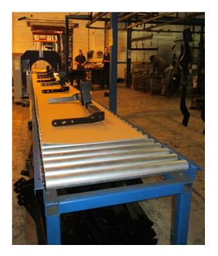
Aetna UK's Robopac Compacta SPR is playing an integral part in A1 Towbar's success story. Individual components are manually picked and placed on a cardboard bed, and they then travel along a roller feed into the wrapping machine itself where they are automatically secured to the bed by stretch wrapping. The ends of the cardboard are folded and the components are placed, as a whole, in a box for final dispatch to the customer.
