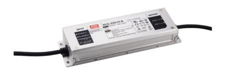
One of the key advantages of the **MEAN WELL XLG-320-V-A** is its dual voltage capability, allowing you to streamline your inventory, and stock only one driver for both 12 volt and 24 volt applications. By selecting the 12 volt option, you can have an output of up to 216 watts, while the 24 volt option provides an output of up to 312 watts.
