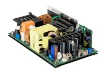
At the heart of this power supply is an impressive 500 watts of output power. The **EPP-500 series** offers exceptional performance with 25CFM forced air cooling, enabling it to deliver 320 watts even under free air convection conditions. Its operating temperature range of -30°C to +70°C ensures reliable performance in various environmental conditions, while the no load power consumption of less than 0.5W demonstrates its energy-efficient design.
