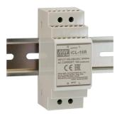
Inrush current is a common problem that occurs when a system powers on and experiences a spike in current, which can be substantially higher than the standard operating current. The ICL-16 series is a reliable solution to this problem. Installing the ICL-16 series inrush current limiter after the AC circuit breaker will significantly reduce the chances of tripping the AC circuit breaker.
