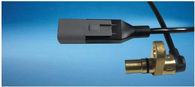
The overmolding of the pre-assembled connector (DEUTSCH DT04 series) creates a perfect, sealed solution. The sensor itself already meets IP6K9K (ISO 20653) and IP67 (EN60529).
